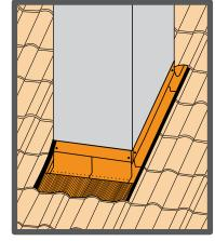
2. waterproofing chimney kit installation diagram on roof tile.
