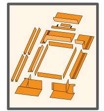
1. Diagram of the different elements waterproofing chimney kit
