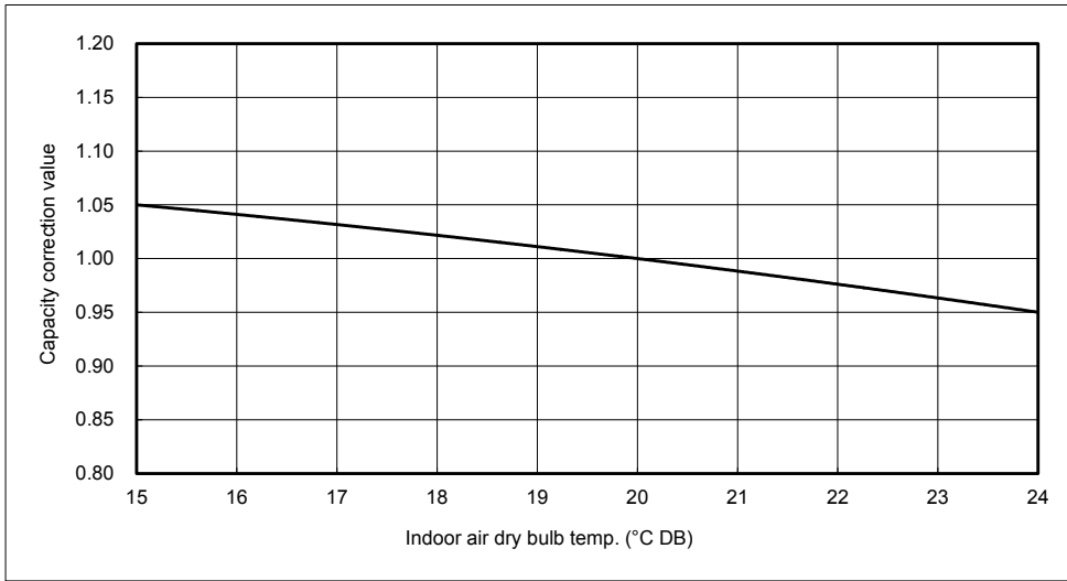
[Chart 1] Indoor air wet bulb temperature vs. capacity correction value
