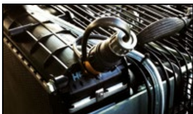
COOLANT LEVEL SENSOR IN RADIATOR.
