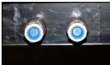
FAST FUEL PLUG CONNECTION BETWEEN EXTERNAL AND INTERNAL FUEL TANK.
