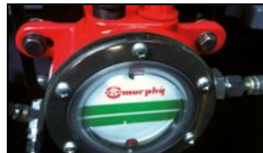
MUR-PHY ENGINE OIL MAINTAINING SYSTEM.
