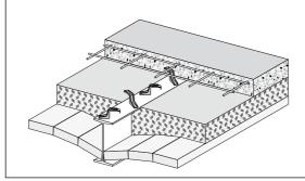
Typical application of X-HVB shear connector with jack arch system (without steel deck), e.g. rehabilitation project.
