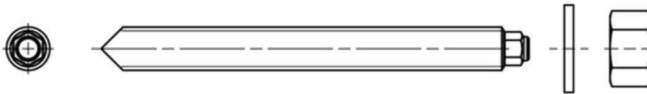
Figure 3: Steel element – threaded rod; 6 mm d \leq 30 mm
