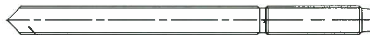
Threaded rod HAS-(E)... thread sizes M8, M10, M12, M16, M20, M24, M27 or M30
