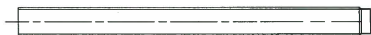
Threaded rod HIT-V-... thread sizes M8, M10, M12, M16, M20, M24, M27 or M30
