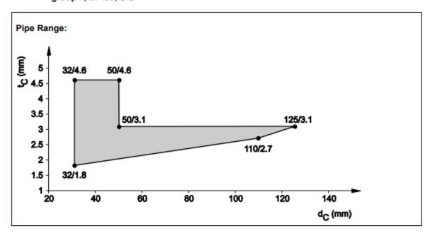
8.4.2.3 PE pipes acc. EN15494, EN 12201-2 and and DIN 8074/75, in rigid wall ( $t_E \ge 100$  mm), pipe group 1, El 120 - U/C
