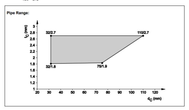
8.3.2.11 PP pipes acc. EN 1451-1 and DIN 8077/78, in flexible wall (t<sub>E</sub> ≥ 100 mm), pipe group 1, EI 120 - U/C
