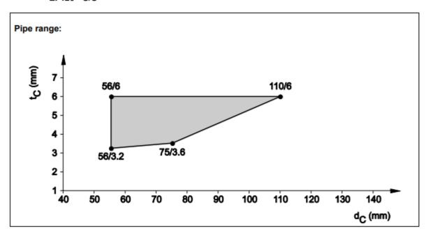
8.5.2.11 PVC-pipes, non-regulated (Friatec Friaphon), in rigid floor (t<sub>E</sub> ≥ 150 mm), pipe group 1, EI 180 - U/U
