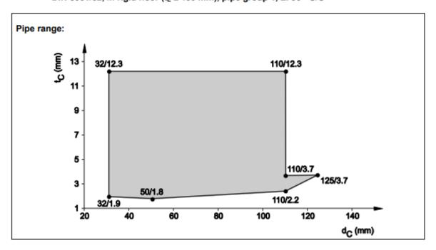
8.5.2.6 PP pipes, non-regulated, pipe types: refer to 8.2.15, in rigid floor (t<sub>E</sub> ≥ 150 mm), pipe group 1, El 120 - U/U
