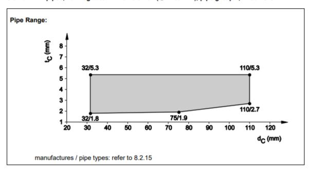
8.3.2.10 PP pipes acc. EN 1451-1 and DIN 8077/78, in flexible wall (t<sub>E</sub> ≥ 100 mm), pipe group 1, EI 120 - U/U
