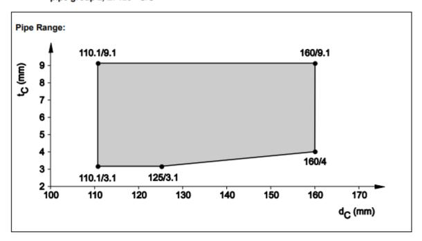
8.4.2.24 PVC pipes acc. EN 1452-1, EN 1329-1, EN 1453-1, EN1566-1, EN ISO 15493 and DIN 8061/62, in rigid wall (t<sub>E</sub> ≥150 mm), pipe group 2, El 120 - U/U
