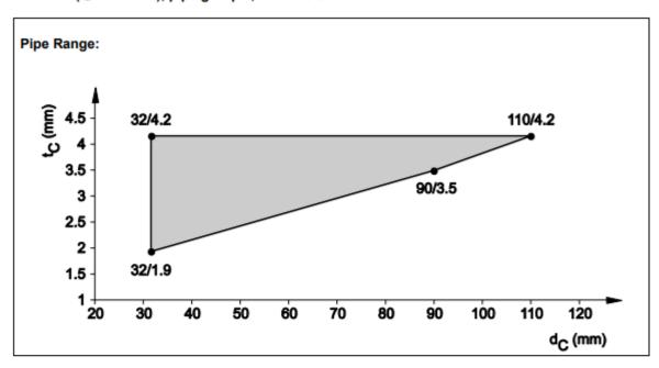
8.3.2.3 ABS- pipes acc. EN 1455, EN 15493 and SAN+PVC-pipes acc. EN 1565-1, in flexible wall, (t<sub>E</sub> ≥ 100 mm), pipe group 1, El 60 - U/U
