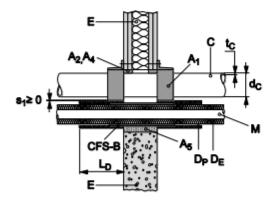
8.3.2.23.2 Pipes in flexible wall (t<sub>E</sub> ≥ 100 mm), pipe group 1, El 90, zero distance between CFS-C EL collar and CFS-B, wrapped around an elastomeric foamed thermal insulation on metal pipe
