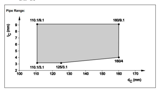
8.4.2.28 PP pipes acc. EN 1451-1 and DIN 8077/78, in rigid wall ( $t_E \ge$  150 mm), pipe group 2, EI 120 - U/C
