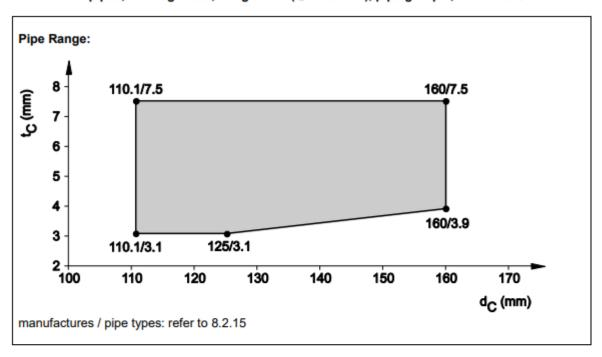
8.4.2.26 PP pipes acc. EN 1451-1 and DIN 8077/78, in rigid wall ( $t_E \ge 150$  mm), pipe group 2, EI 120 - U/U
