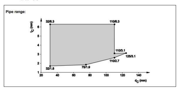
8.5.2.9 PP pipes acc. EN 1451-1 and DIN 8077/78, in rigid floor ( $t_E \ge$  150 mm), pipe group 1, EI 120 - U/C
