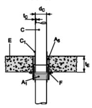
8.5.2.15 PE pipes acc. EN 1519-1, EN 12201-2 and EN 12666-1, in rigid floor (t<sub>E</sub> ≥ 150 mm), pipe group 2, El 120 - U/U
