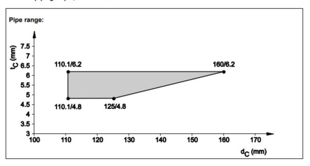
8.5.2.16 ABS pipes acc. EN 1455-1, EN 15493 and SAN+PVC-pipes acc. EN 1565-1, in rigid floor (t<sub>E</sub> ≥ 150 mm), pipe group 2, El 120 - U/U
