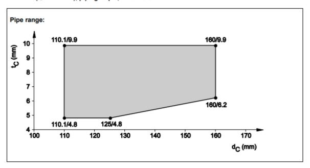
8.5.2.18 PE pipes acc. EN 15494, EN 12201-2 and DIN 8074/75, in rigid floor (t<sub>E</sub> ≥ 150 mm), pipe group 2, EI 90 - U/U
