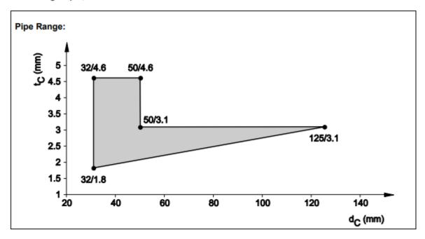
8.3.2.5 PE pipes acc. EN 15494, EN 12201-2 and DIN 8074/75 in flexible wall, ( $t_E \ge 100$  mm), pipe group 1, EI 90 - U/U
