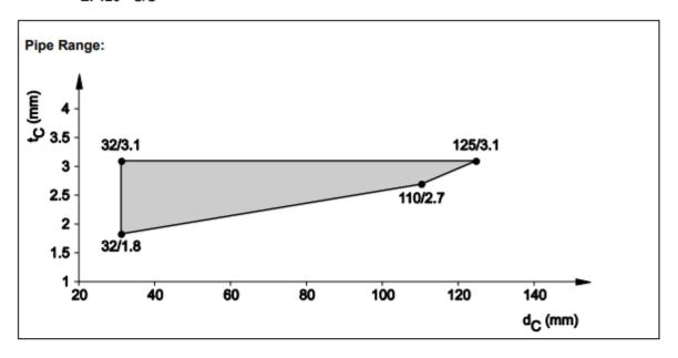
8.4.2.7 PP pipes acc. EN1451-1 and DIN 8077/78, in rigid wall (t<sub>E</sub>  $\geq$  100 mm), pipe group 1, EI 120 - U/C
