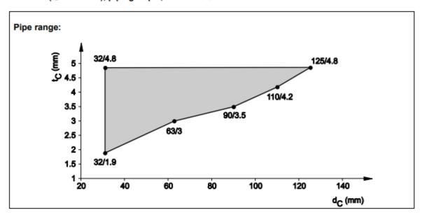
8.5.2.3 PE pipes acc. EN 15494, EN 12201-2 and DIN 8074/75 in rigid floor (t<sub>E</sub> ≥ 150 mm), pipe group 1, El 120 - U/U
