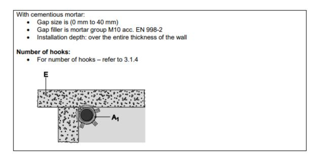
8.4.2.20 PE pipes acc. EN 1519-1, EN 12201-2 and EN 12666-1, in rigid wall (t<sub>E</sub> ≥ 150 mm), pipe group 2, El 120 - U/U
