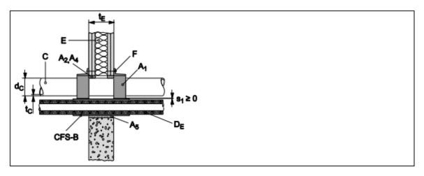
PE foamed insulation or PE protection tube on aluminum composite EI90 U/C
