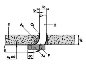
8.5.2.48 PVC pipes acc. EN 1452-1, EN 1329-1, EN 1453-1, EN 1566-1; DIN 8061/62, EN ISO 15493 in rigid floor (t<sub>E</sub> ≥ 150 mm), pipe group 1, El 120 - U/U, Pipe Elbow 87°
