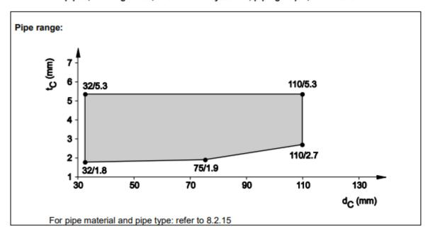
8.6.2.5 PP pipes acc. EN 1451-1 and DIN 8077/78, in shaft wall system A, pipe group 1, EI 90 - U/U
