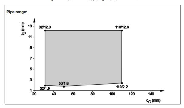
8.5.2.5 PVC pipes acc. EN 1452-1, EN 1329-1, EN 1453-1, EN 1566-1, EN ISO 15493 and DIN 8061/62, in rigid floor (t<sub>E</sub> ≥ 150 mm), pipe group 1, EI 90 - U/U
