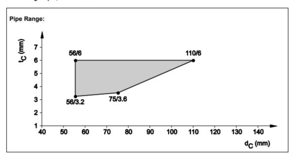
8.3.2.13 PVC- pipes, non-regulated (Friatec Friaphon), in flexible wall (t<sub>E</sub> ≥ 100 mm), pipe group 1, EI 90 - U/U
