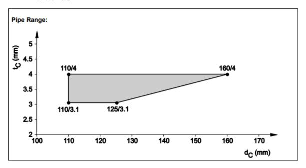
8.4.2.27 PP pipes acc. EN 1451-1 and DIN 8077/78, in rigid wall ( $t_E \ge 150$  mm), pipe group 2, EI 30 - U/U
