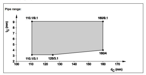
8.5.2.19 PE pipes acc. EN 15494, EN 12201-2 and DIN 8074/75, in rigid floor ( $t_E \ge$  150 mm), pipe group 2, EI 120 - U/C
