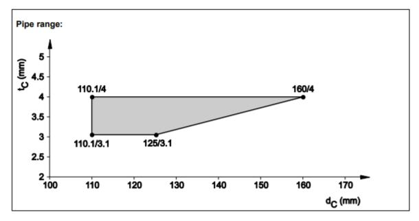
8.5.2.21 PVC pipes acc. EN 1452-1, EN 1453-1, EN 1566-1, EN 1329-1, EN ISO 15493 and DIN 8061/62, in rigid floor (t<sub>E</sub> ≥ 150 mm), pipe group 2, El 90 - U/U
