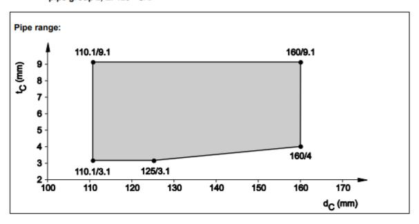
8.5.2.20 PE pipes acc. EN 15494, EN 12201-2 and DIN 8074/75, in rigid floor (t<sub>E</sub> ≥ 150 mm), pipe group 2, El 120 - U/U
