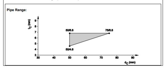
8.4.2.17 PP pipes, non-regulated, gap sealed with CFS-FIL, in rigid wall (t<sub>E</sub> ≥ 100 mm), pipe group 1, El 90 - U/U, elbow pipe 87°
