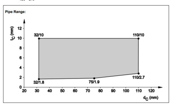
8.3.2.12 PE pipes, non-regulated (Geberit Silent dB20), in flexible wall (t<sub>E</sub> ≥ 100 mm), pipe group 1, El 120 - U/U
