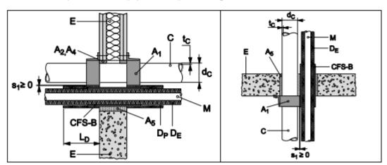
In floor application (t<sub>E</sub> ≥ 150 mm) there is no need for an additional protect insulation D<sub>P</sub>.
