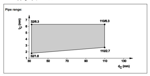
8.6.2.3 PVC pipes acc. EN 1452-1, EN 1329-1, EN 1453-1, EN 1566-1, EN ISO 15493 and DIN 8061/62, in shaft wall system A, pipe group 1, El 90 - U/U
