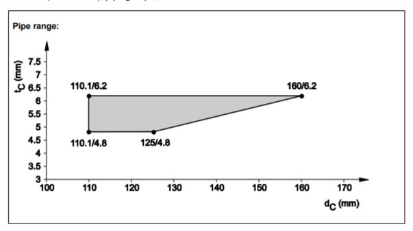
8.5.2.17 ABS pipes acc. EN 1455-1, EN 15493 and SAN+PVC-pipes acc. EN 1565-1, in rigid floor (t<sub>E</sub> ≥ 150 mm), pipe group 2, El 60 - U/U
