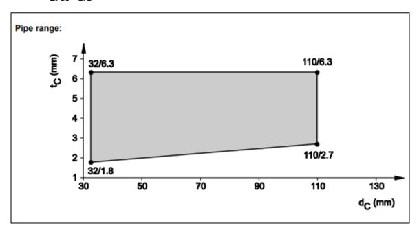
8.6.2.6 PE pipes non-regulated (Geberit Silent dB20), in shaft wall system A, pipe group 1, EI 90 - U/U
