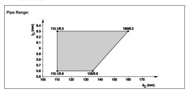
8.5.2.28 PE-X - pipes acc. EN 15875 (Rehau Rautitan flex), insulated, in rigid floor (t<sub>E</sub> ≥ 150 mm), pipe group 1, El 120 - U/C
