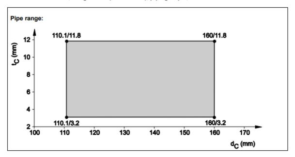
8.5.2.22 PP pipes, non-regulated, in rigid floor (t<sub>E</sub> ≥ 150 mm), pipe group 2, El 120 - U/U
