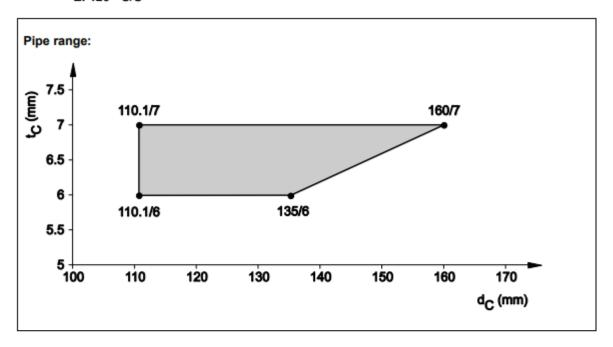
8.5.2.26 PVC pipes acc. EN 1452-1, EN 1329-1, EN 1453-1, EN 1566-1, EN ISO 15493 and DIN 8061/62, in rigid floor (t<sub>E</sub> ≥ 150 mm), pipe group 2, El 120 - U/C situation
