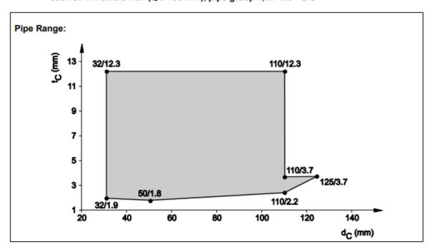
8.3.2.9 PP pipes, non-regulated in flexible wall (t<sub>E</sub> ≥ 100 mm), pipe group 1, El 90 - U/U
