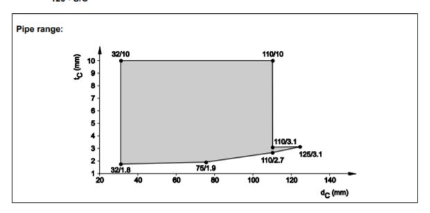
8.5.2.10 PE pipes, non-regulated (Geberit Silent dB20), in rigid floor (t<sub>E</sub> ≥ 150 mm), pipe group 1, EI 120 - U/U
