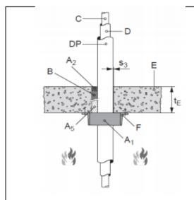
Wavin Tigris PE-X-One R-I-R insulated, penetrating a rigid floor
