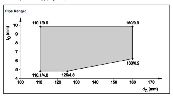
8.4.2.22 ABS pipes acc. EN 1455-1, EN 15493 and SAN+PVC-pipes acc. EN 1565-1, in rigid wall (t<sub>E</sub> ≥ 150 mm), pipe group 2, El 120 - U/C
