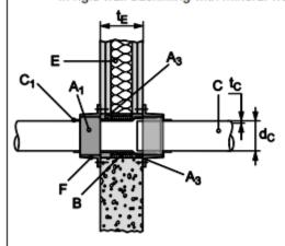
Requested number of hooks on CFS-C EL to seal pipes, penetrating a flexible wall/ rigid wall ( $t_E \ge 100$ mm) and using a linear pipe coupling. (no elbow). If pipe insulation thickness is between 0 and 4 mm use the number of hooks indicated for 4 mm. If pipe insulation thickness is between 4 and 9 mm use the number of hooks indicated for 9 mm.
