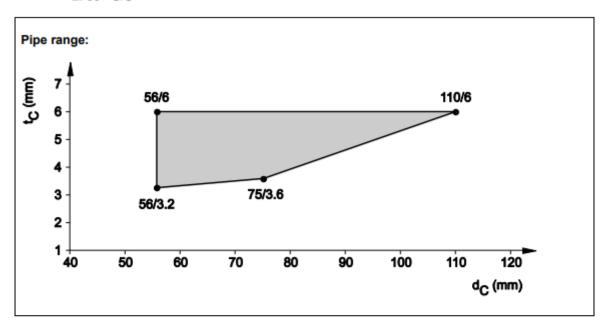
8.6.2.7 ABS pipes acc. EN 1455-1, EN 15493 and SAN+PVC-pipes acc. EN 1565-1, in shaft wall system A, pipe group 1, EI 90 - U/U
