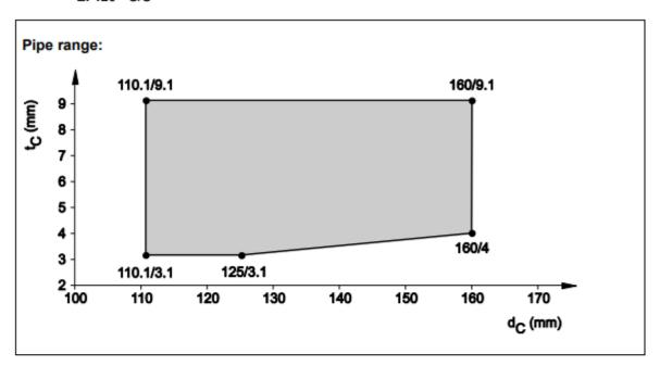
8.5.2.24 Pneumatic dispatch system, PVC-U pipes acc. DIN 6660, in rigid floor (t<sub>E</sub> ≥ 150 mm), pipe group 2, El 120 - U/U, straight (90°) installed
