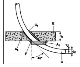
8.5.2.13 PE pipes, non-regulated (Geberit Silent dB20), in rigid floor (t<sub>E</sub> ≥ 150 mm), pipe group 1, EI 120 - U/U, straight (90°), 2 x 45° elbow pipe connector
