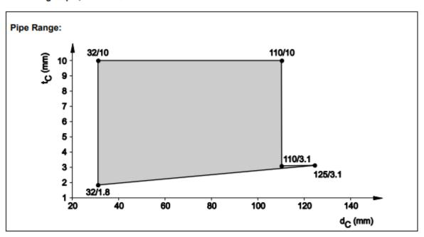
8.3.2.7 PE pipes acc. EN 15494, EN 12201-2 and DIN 8074/75 in flexible wall (t<sub>E</sub> ≥ 100 mm), pipe group 1, EI 90 - U/C
