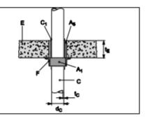
Plastic pipe, penetrating a rigid floor, sealed with Hilti Firestop Collar Endless CFS-C EL. Used gap filler is CFS-S ACR in a thickness of (t<sub>A2</sub> ≥ 25 mm) from the upper surface of the floor only, backfilled with mineral wool.
