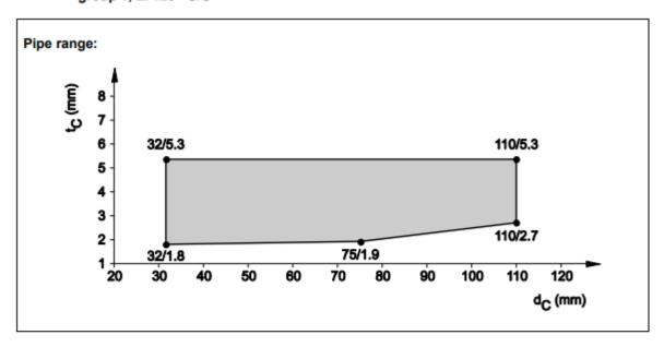
8.5.2.7 PP pipes acc. EN 1451-1 and DIN 8077/78, in rigid floor (t<sub>E</sub> ≥ 150 mm), pipe group 1, EI 120 - U/U
