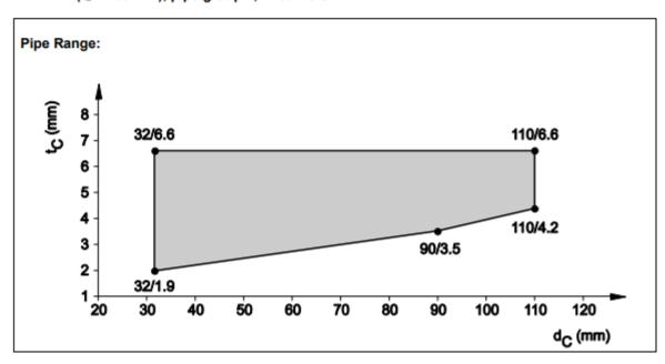
8.3.2.4 PE pipes acc. EN 15494, EN 12201-2 and DIN 8074/75 in flexible wall, (t<sub>E</sub> ≥ 100 mm), pipe group 1, El 120 - U/U
