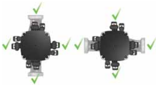
Fig. 22 Possible control box positions
