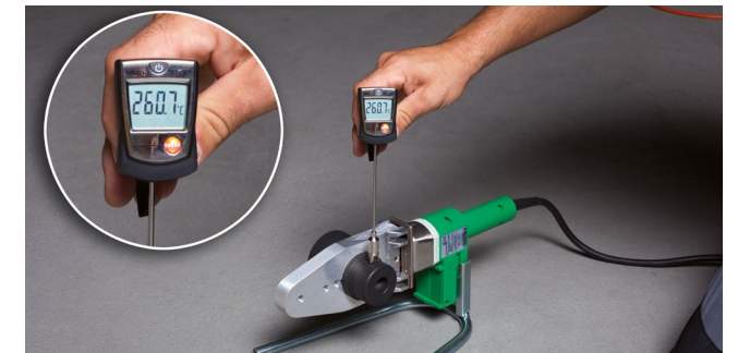
Measurement of temperature with the aquatherm manual welding device (800 W).
