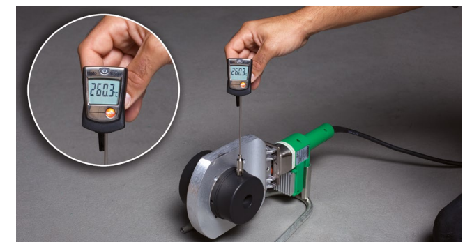
Temperature control aquatherm welding device (1400 W)
