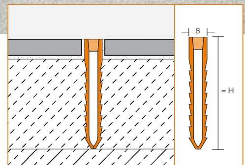
Schlüter®-DILEX-MOP is installed as a movement joint in tiled surfaces set into a mortar bed. Individual covering fields are separated by the profile whose soft PVC movement zone equalizes compressive stresses.
