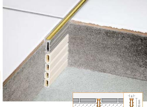
The profiles with inserts of brass or chrome material are coated with a protective layer of transparent PVC. The bottom section of the profile consists of detachable segments made of soft PVC. The upper side walls feature dove-tailed ribs for anchoring the profile to the mortar bed.
