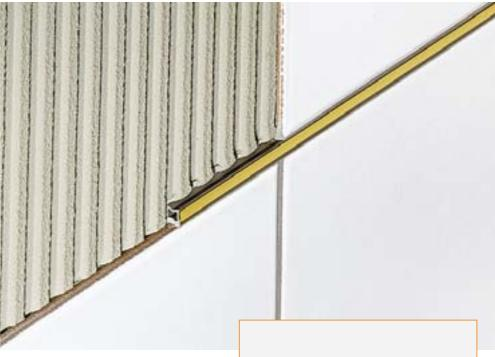
Schlüter<sup>®</sup>-DILEX-EZ 6 and -EZ 9 are decorative expansion joints used with tiled surfaces. Two soft PVC surfaces connect and overlap rigid PVC side sections at the top and bottom in two different colours, creating two usable surfaces which absorb compressive stresses.
