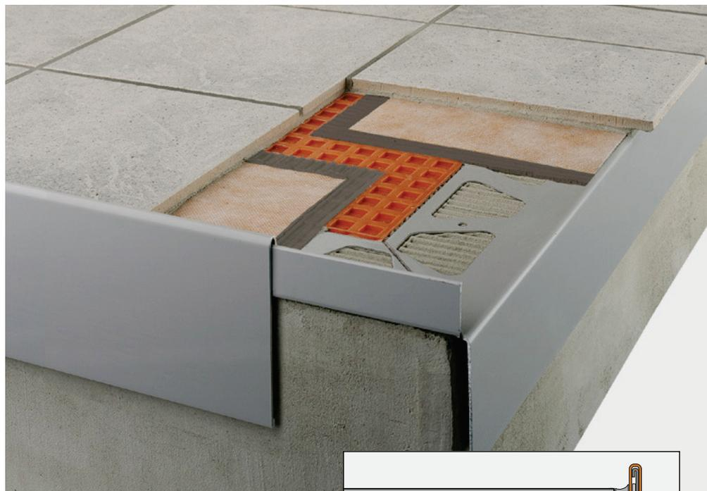
All cavities of the setting material for embedding Schlüter®-BARA-RW must be filled to prevent the collection of water, since water with a high alkaline concentration can corrode the aluminium.
